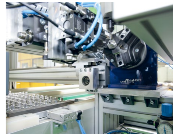
Labelling of pressure-bearing components
