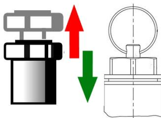
Step 1: Pull the lifting knob / pull-ring upwards until blow-off of the operating medium is clearly audible.
