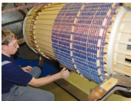
Particular care has to be taken when producing the windings of a transformer
